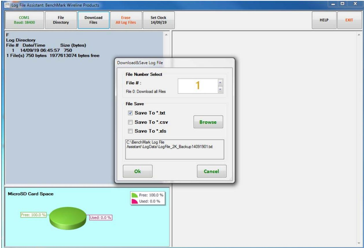
Clicking on the 'Download Files' button will open a new dialog window. A specific log file is then chosen from the list box and the Operator has the option of saving the file in three different file extension formats; and re-naming and re-locating the file using the 'Browse' button.
