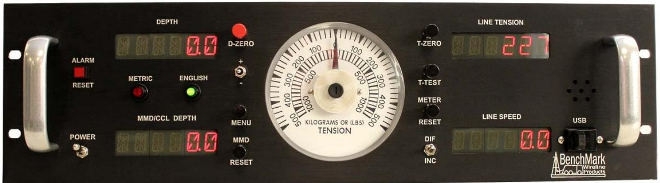
Depth is displayed from data provided from an encoder mounted on a measuring device. The encoder quadrature pulses are passed through to the acquisition system. The tension data is provided by a load pin and is also passed through to the acquisition system.
