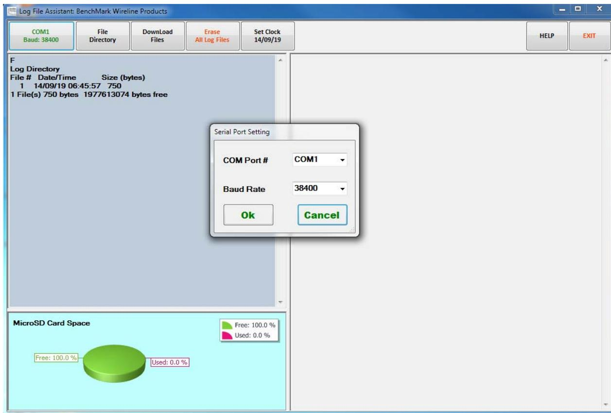
Upon program start the available laptop computer COM Ports are searched for availability. If the COM Port button text reports that no connection is made, click on the button and then pull down the COM Port # list box and choose the proper COM Port.
