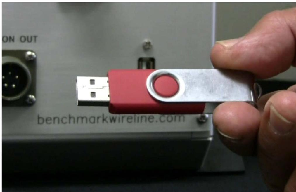
Go to the BenchMarkWireline.com website and then Support and Software Downloads. Insert the memory stick in that computer. On the memory stick make a new folder named "ams2000" in lower case. Locate the software update file for your panel. Then download the file into the new folder on the memory stick. Then rename the downloaded file "ams2000.hex" all lower case.
