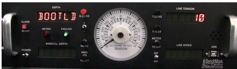
When it hits zero, the panel will automatically erase the current software on the panel. It will also automatically upload the necessary files from the memory stick to the panel. This may take up to 5 minutes.
