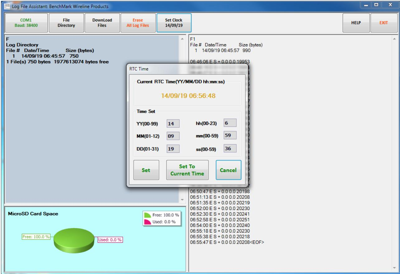
Clicking on the 'Set Clock' button will open a dialog that allows the Operator to set the Date/Time clock to the current Date/Time or to any Date/Time desired.
