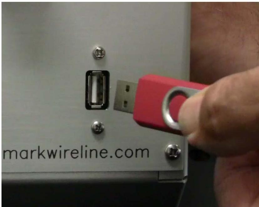
Now Power ON the panel and it will go through an automatic boot cycle. Very quickly it will recognize the presence of the memory stick and will begin a 10-0 countdown on the Line Tension screen.
