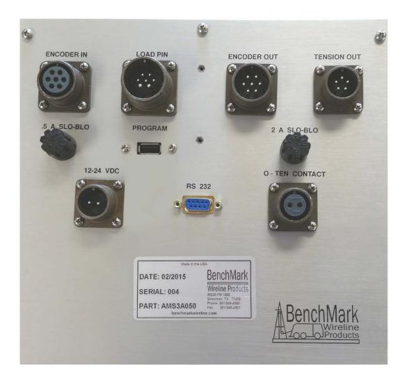
Depth is displayed from data provided from an encoder mounted on a measuring device. The encoder quadrature pulses are passed through to the acquisition system. The tension data is provided by a load pin and is also passed through to the acquisition system.
