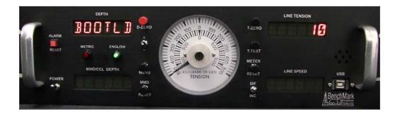
When it hits zero, the panel will automatically erase the current software from memory.. It will also automatically upload the necessary files from the memory stick to the panel. This may take up to 5 minutes.
