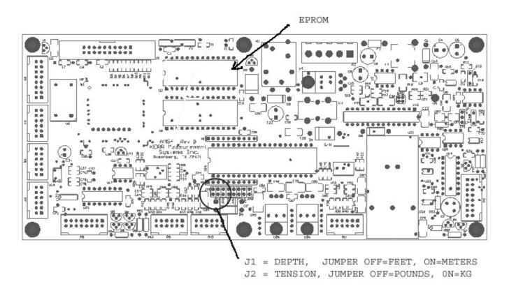
Jumpers are used to select default depth and tension units as well as Head Type and Load Pin type.. These units can also be set with the menu commands (see section 3) but when the panel is rebooted, it will be reset to the Jumper settings.
