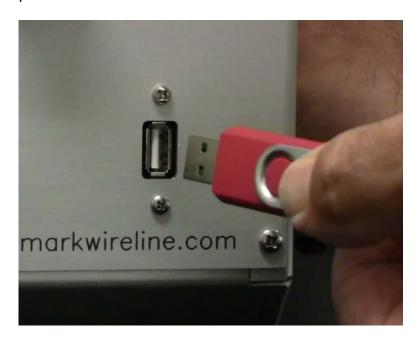
Now Power ON the panel and it will go through an automatic boot cycle on the **Depth Display**. Very quickly it will recognize the presence of the memory stick and will begin a 10-0 countdown on the **Line Tension** display. Note – these 2 displays may be in different positions on your panel.
