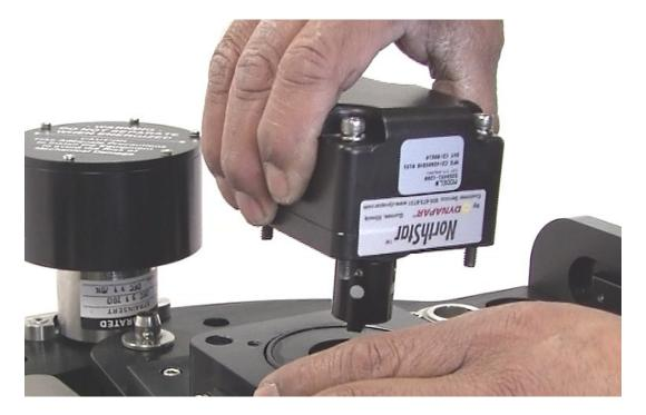
Remove the plug on the encoder adapter body. This may take a big wrench.
