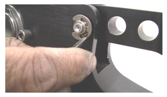
Now remove the pivot pin. You'll have to press down on the spring end of the bar to allow the pin to come free.
