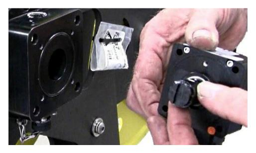
Carefully position the encoder in the adapter body.
