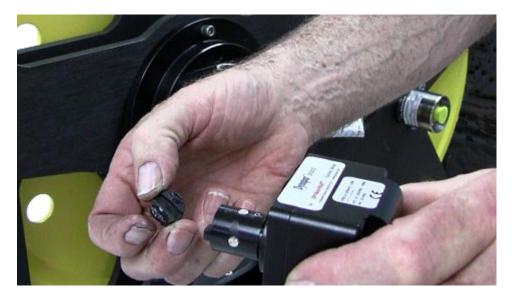
Note the size of the gap between the coupling and the encoder body.
