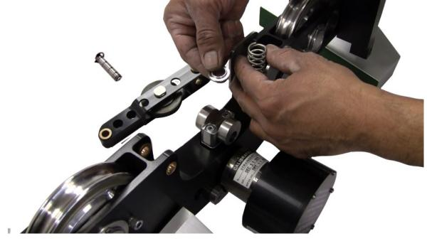
Position the bar as shown in the picture first with the tail of the beam inserted under the metal bar on the right. Then push down on the beam so the pivot pin on the left can be passed through bar and frame.
