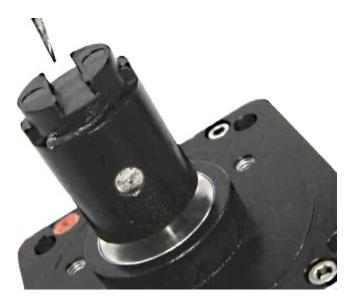
Look through the hole in the adapter body and you will see the coupling half. Rotate the measuring wheel so that the tang on the coupling half is vertical.
