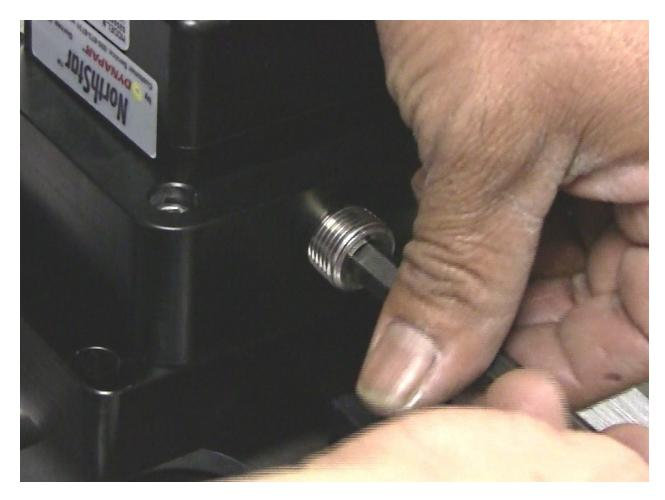
Replace the plug in the encoder adapter. Use Teflon tread tape and tighten the plug firmly.
