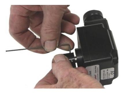
Lubricate the O ring using the DC111 and carefully replace the O ring in the adapter body.
