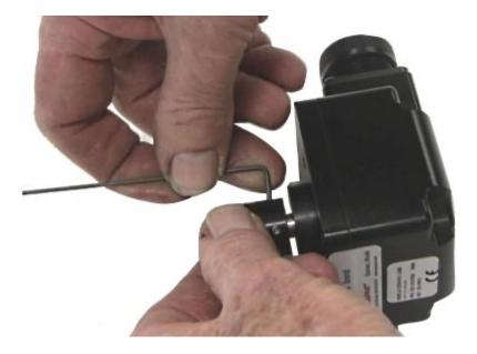
Remove the coupling stack from the shaft.
