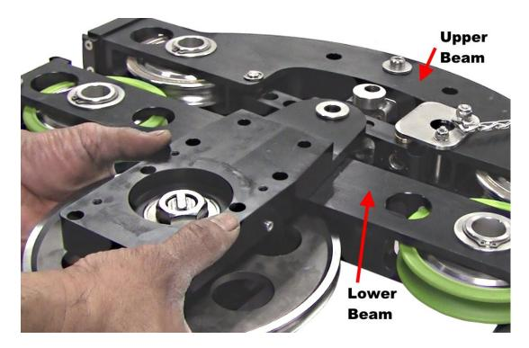
Slide the side panel/wheel assembly with the nut side up, back onto the measuring head frame which should be positioned encoder side down.
