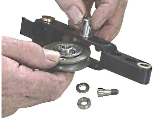
Some adjustment and pressure may be necessary as the lock washer must fit into notch in the wheel. Tighten the screw firmly.
