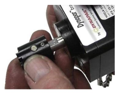
When tightening, leave the same gap on the shaft between the coupling and the encoder. Snug up but DO NOT fully tighten the set screw on the flat side of the shaft.
