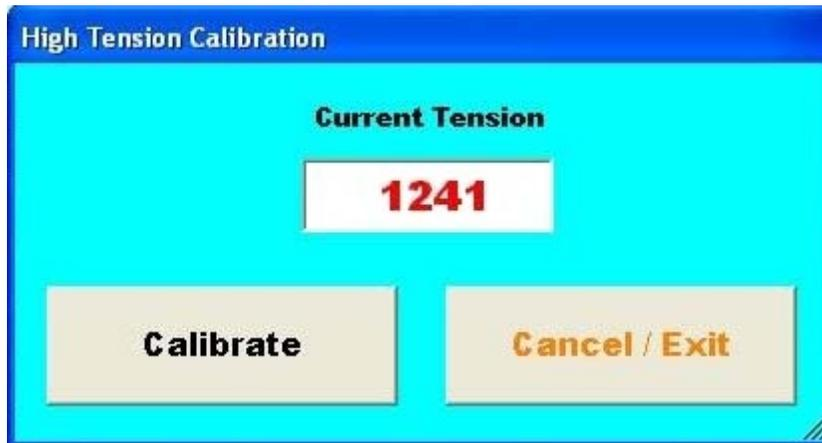
Pressing Tension Cal will activate the tension relay inside the panel. The load pin should then return a calibrated signal that varies depending on the head chosen.
