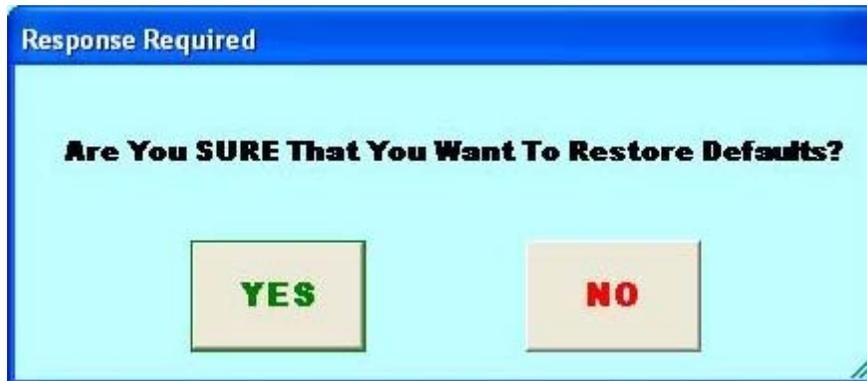
When this button is pressed, all the settings will be restored to their default values. This functions as a software reset. Depth will be zeroed.
