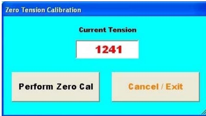
Pressing Tension Zero will null out any tension offset voltage up to 200 lbs (slickline head) or 1000 AM5K braided line head.
