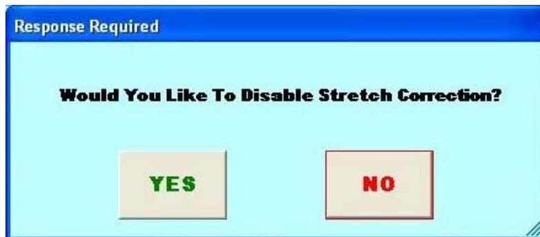
Enabling this allows stretch correction to automatically be applied to the depth. The correction is calculated using line size and mud cable coef. parameters
